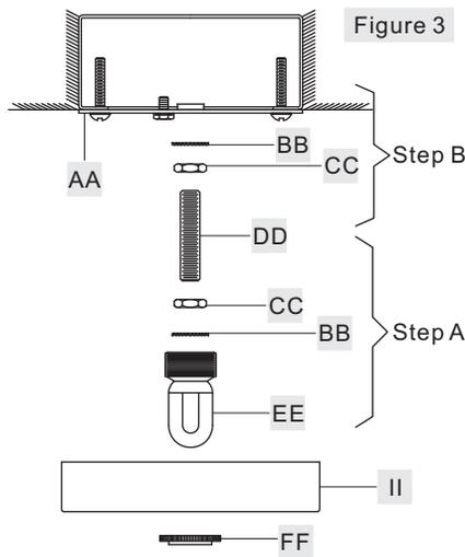
**STEP 4 - Install Fixture Chain and Ceiling Canopy**
