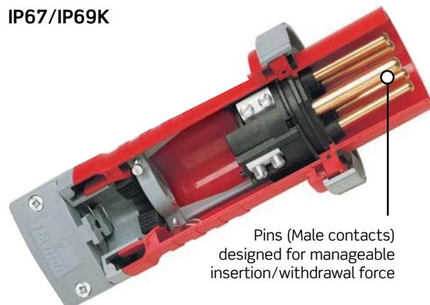
Pins (Male contacts) designed for manageable insertion/withdrawal force
