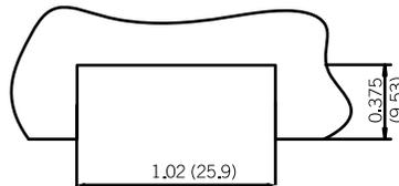
Recommended Panel Opening for Miniature Bi-Pin Snap-In/Slide-On Lampholders
