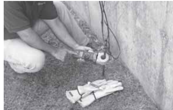
The DET20C being used to test a facility ground.
