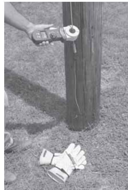
The DET20C being used to test a pole ground.
