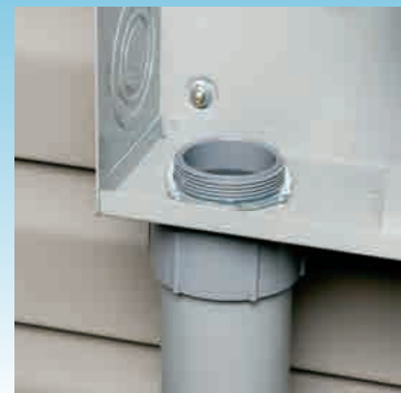
Attach the NM2520 to the bottom of the meter enclosure. 2 to 2-1/2" meter riser fitting holds conduit firmly in place (locknut is not supplied).
