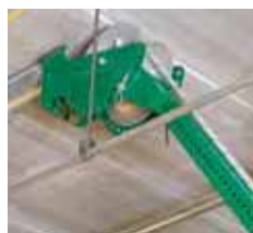
Optional 12' boom extension for high pulls
