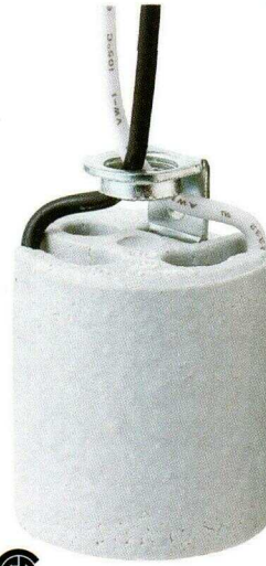
FIXTURE 22370 - 10" WIRE LEADS STANDARD BASE 3/8-IP HICKEY 18 GAUGE, 105'LEADS 660 WATTS 250 VOLTS HEIGHT - 2"
